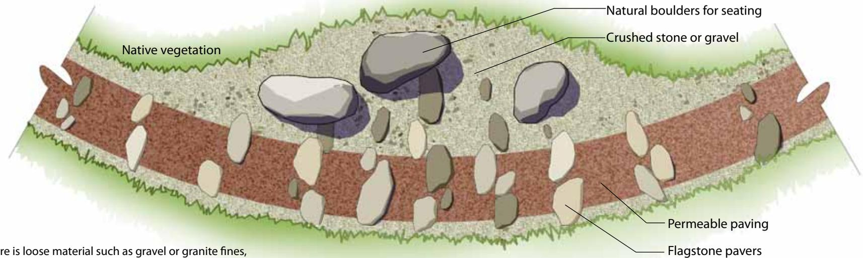
Note: If there is loose material such as gravel or granite fines, then an edge restraint (such as steel edging) is required to contain the material.
