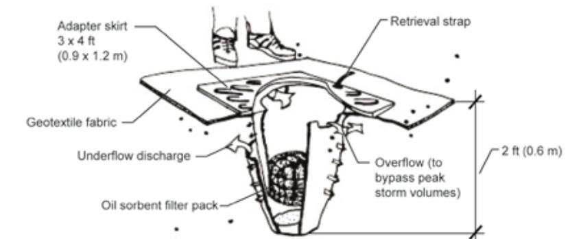
Diagram of a stormwater catch basin insert
