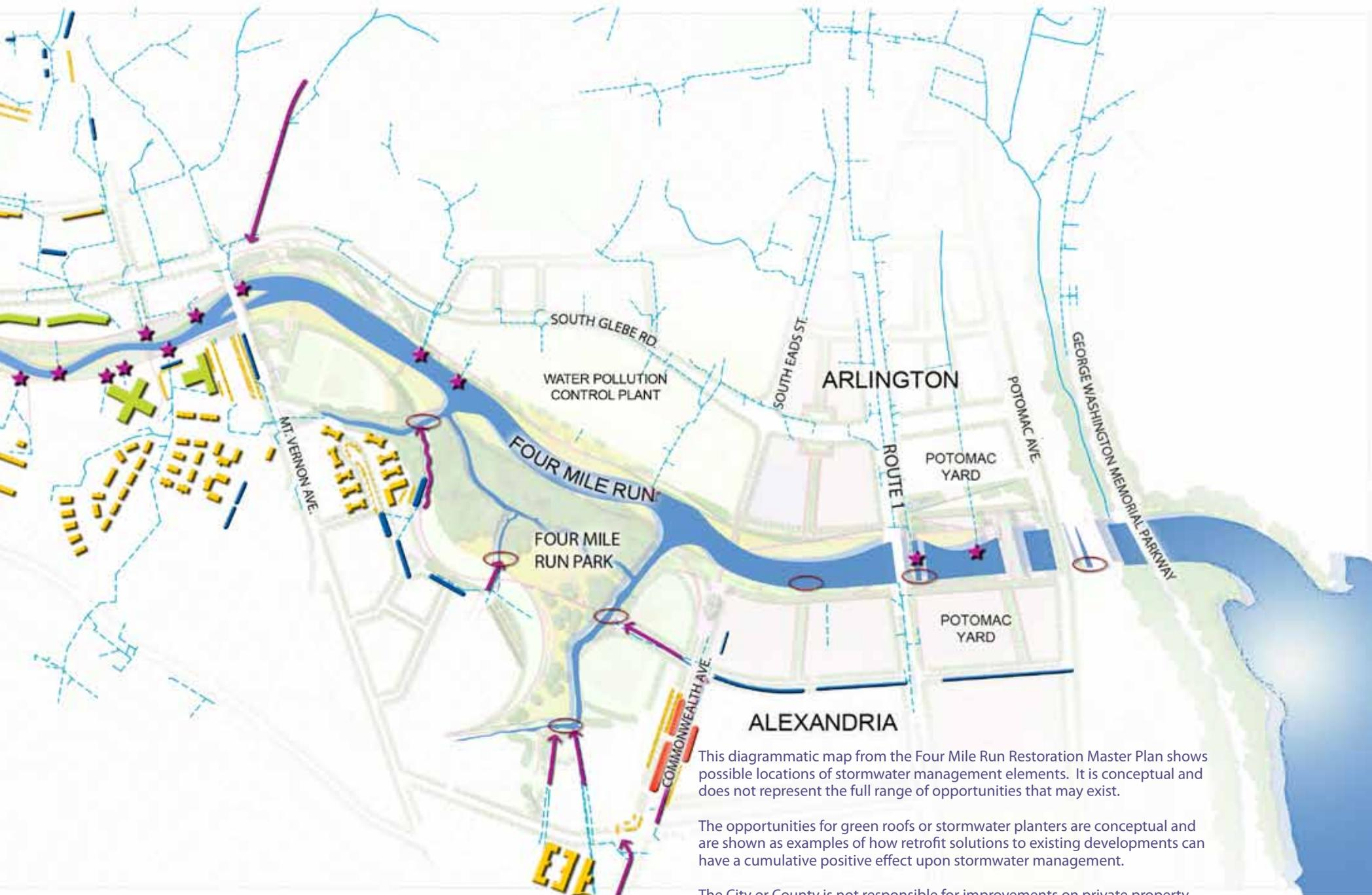
This diagrammatic map from the Four Mile Run Restoration Master Plan shows possible locations of stormwater management elements. It is conceptual and does not represent the full range of opportunities that may exist.
