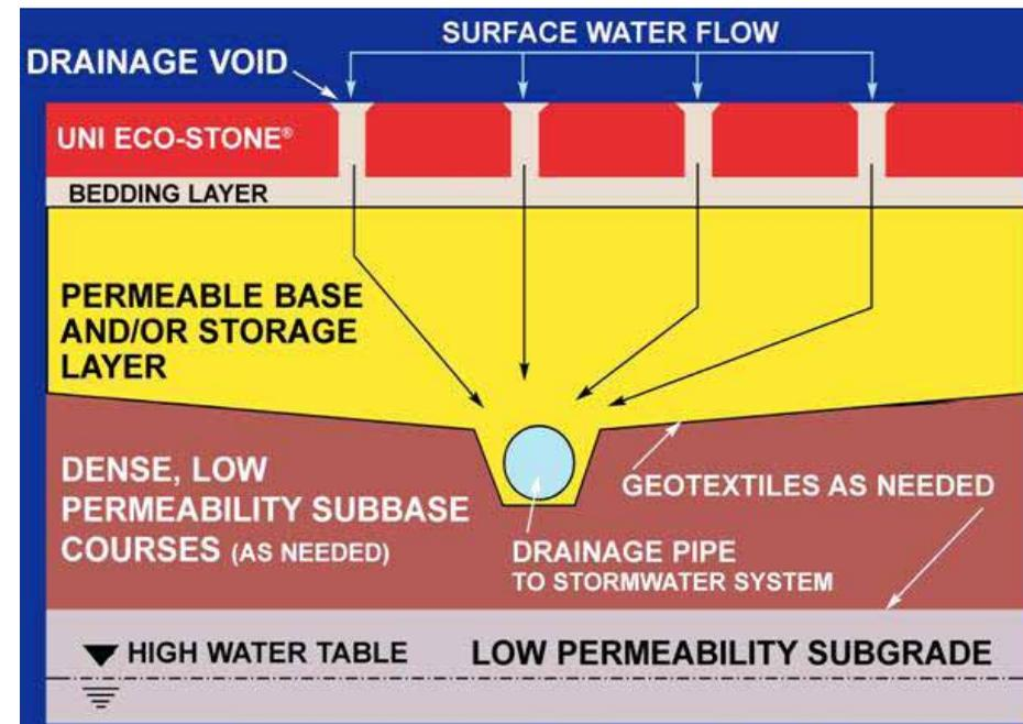
Typical permeable paving section
