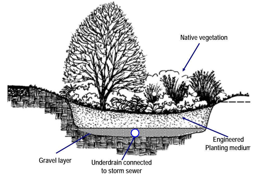
Typical bioretention detail
