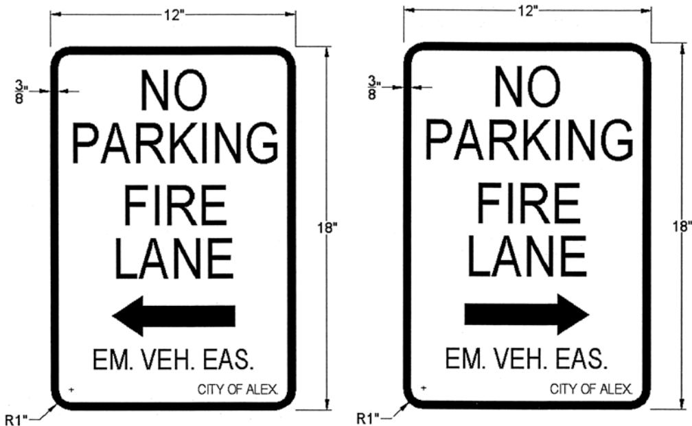
Fire Lane Sign Left Arrow Fire Lane Sign Right Arrow
